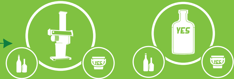
Bottles are placed into the Sbriciola glass crusher and are reduced to 1/10 of their original volume in just 5 seconds..
